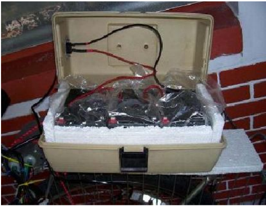
Enclosure for lead acid batteries made from plastic tool box and fitted with connector.
